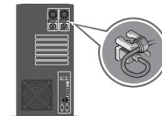
**4** **Loop and secure the power cable using the retention clip.**
